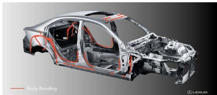
*Figure 1 - Adhesives were used to join body panels over a larger area to make significant improvements to body rigidity*
